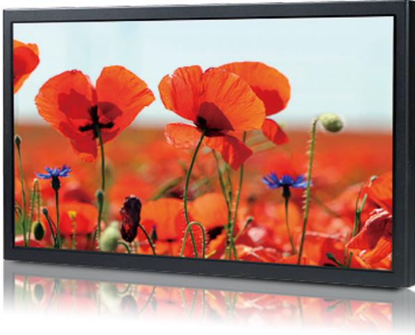
MPPC 2120T is a 21.5" wide 16:9 touch screen Panel PC which can display resolutions up to 1920 x 1080 (Full HD). Based on the Atom™ D525, MPPC 2120T has low power consumption and a totally fanless design.
